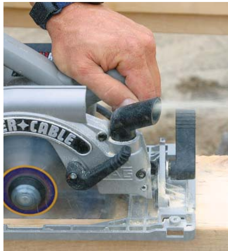
Top marks for dust control. The adjustable dust port on the Porter-Cable saw lets you blow sawdust in any direction, back into the blade housing, or into a shop-vacuum hose.
