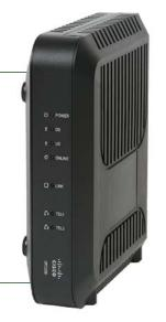
WAP A wireless access point (WAP) is connected to a router and transmits a wireless signal; 802.11ac is the most recent wireless communication standard. Dual-band WAPs can communicate with both 2.4-GHz and 5-GHz devices at once, which means less interference and a more reliable signal.
