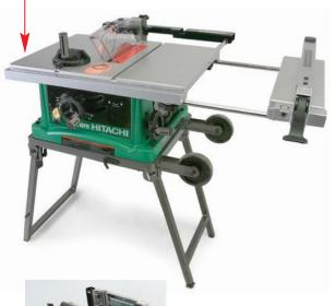
A low handle forces you to stoop when rolling the saw, and the small plastic wheels are a poor substitute for the large rubber wheels found on other saws. Onboard storage is good.
