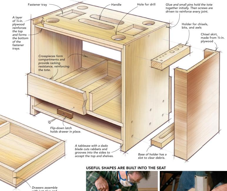
Drawers assemble with just glue and brads. Put in only a couple of dividers so that the drawer can hold larger items.
