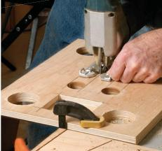
**Holes and a handle.** Lay out the top of the tote (or the seat) with a comfortable handle, holes for tools such as drills, and trays for fasteners. A hole saw makes a place for a drill, and a jigsaw cuts the handles.
