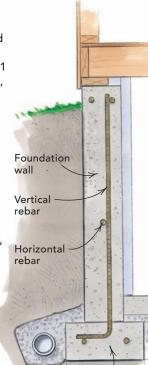
Best-practice solution: Consult the seismic map in the IRC to determine whether you need rebar in foundation walls. But remember, rebar is cheap insurance.
