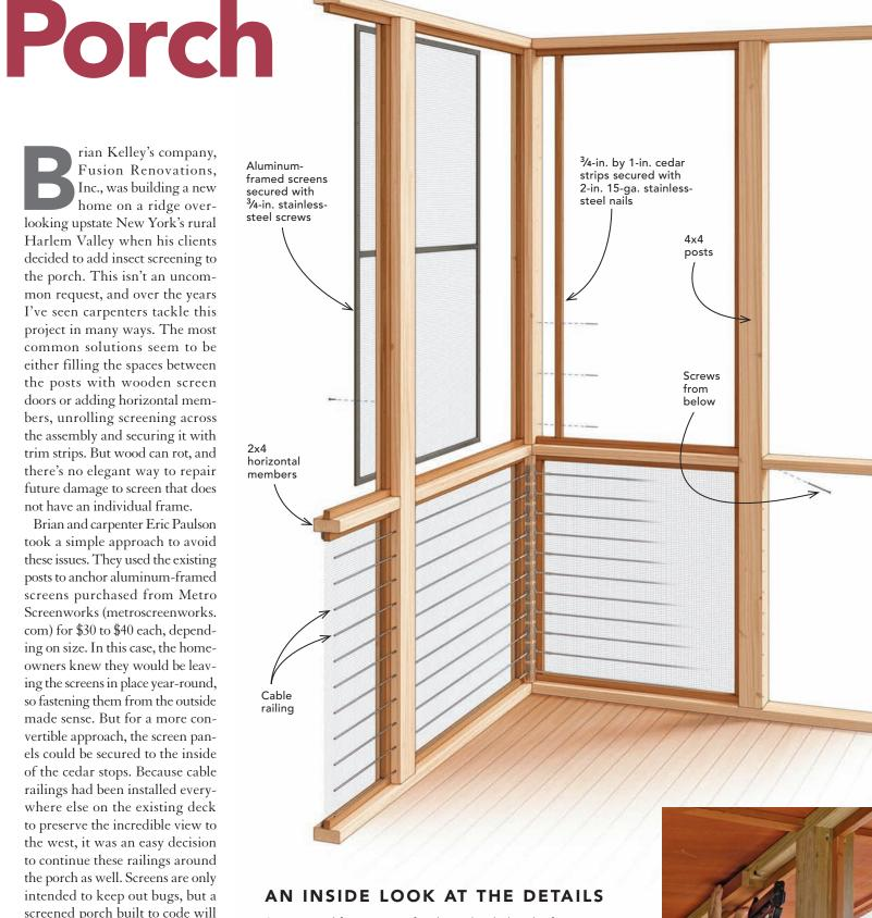
Stops ripped from scraps of cedar and nailed to the framing create attachment points for the screens. A spacer block is used to locate the strips consistently. Stainless-steel screws fasten the screens to the mounting strips. The screens are easily removed should one need repairs. If seasonal removal of the screens had been desired, the screens could have been mounted from inside for easier removal.
