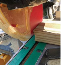
Birdsmouth bevels. The angled baluster ends look tricky, but are easy to cut on a sliding miter saw. Use a stop to ensure that each baluster is the same length, set the saw to a 7° bevel angle, and set the saw's cutting-depth stop to limit the blade depth to half the thickness of the stock. The birdsmouth is then made in two cuts that meet in the middle.
