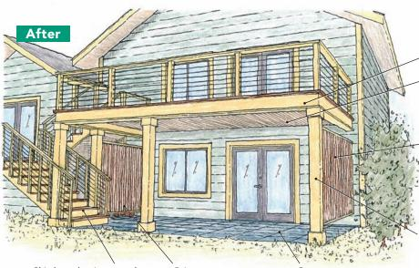
Skirtboards, risers, and railings give the deck stairs a level of finish similar to that of an indoor stair.
