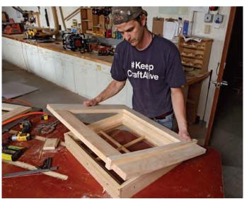
Spacers set the sash. Cut the jamb stock to be just a whisker larger than the sash, then fasten the jambs together with countersunk screws before dropping the sash into place. Use spacer blocks to support and locate the sash, then secure it with screws through the back of the jambs.
