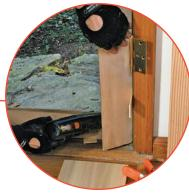
Secure the template with hot-melt glue. Pull apart each overlapping strip, apply the glue, and replace the clamp. In a minute or two, you can remove the template and place it on the door.
