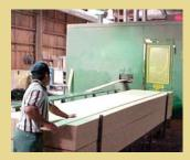
DF is made of a wood-fiber and resin mixture that's compressed into long, flat sheets. After the sheets are ripped into appropriate widths, they're run through a molding machine to form the profile. High-density MDF trim is a smart choice in high-traffic locations and for long, straight runs. Lower-density products are lighter weight, but they aren't as durable and don't hold fasteners as well. Many local and regional lumberyards purchase or mill their own MDF trim, but several manufactur-
