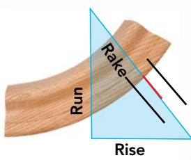
**2 Level-to-rake cut:** For this cut, the pitch-block orientation is reversed.
