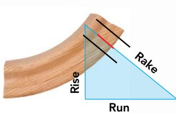
**1 Rake-to-plumb cut:** The cut location is the point (tangent) where the pitch block (with the "Rise" side down) touches the curve of the easement. Because it is difficult to see exactly where the straight line and the curve meet, identify the range where they could touch (black lines), and mark the middle (red line). To mark the cut angle, reorient the pitch block so that the "Run" side is down.
