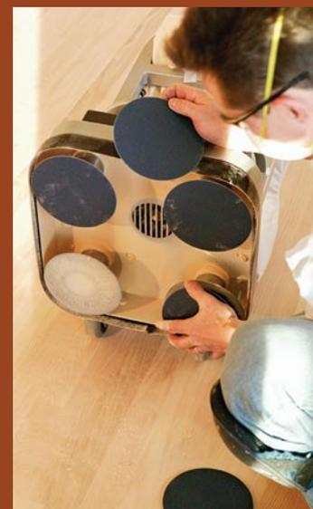
**Foolproof operation, professional results.** The four orbiting heads on the U-Sand rental machine can handle every aspect of floor sanding and eliminate the possibility of gouging the floor.
