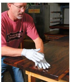
Wet-sand the last coat. When the counter stops absorbing the finish at a dramatic rate, likely by the third coat, apply the finish, and wet-sand it with fine foam sanding pads.
