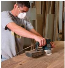
Sand, then sand more. With 60-grit sandpaper on a random-orbit sander, correct any cosmetic defects, paying special attention to the joints. Use a straightedge to make sure that the top is perfectly flat. Sand with 80-, 100-, 120-, and 180-grit sandpaper. Start sanding the edges once you've gotten to the 120-grit paper. Wet the top with mineral spirits to reveal remaining defects.
