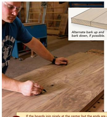
Lay out for looks first. Pick the best face of each board, and lay the boards side by side. To help keep the top flat over time, try to arrange them so that they alternate bark up and bark down (drawing above). But don't sacrifice a perfect face for a top that will be well fastened to the cabinets. Draw a triangle across all the boards to maintain the arrangement.
