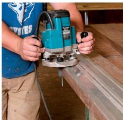
**Prepare the surfaces' mating edges.** Use a jointer or a router and guide to create one perfectly straight edge. If you use the latter technique, rip the board on a tablesaw, removing just enough material to create a parallel straight edge. Flatten the board on a jointer, and plane it to within ½2 in. of final thickness. The remaining ½2 in. will be removed later when the blank is sanded.
