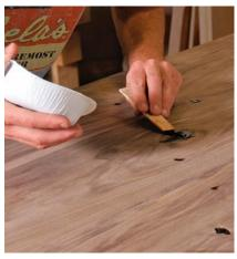
Fill knots and blemishes with epoxy. After scraping away any loose material, use five-minute epoxy with a coloring dye (www.homestead finishingproducts.com) to fill knots and other blemishes.
