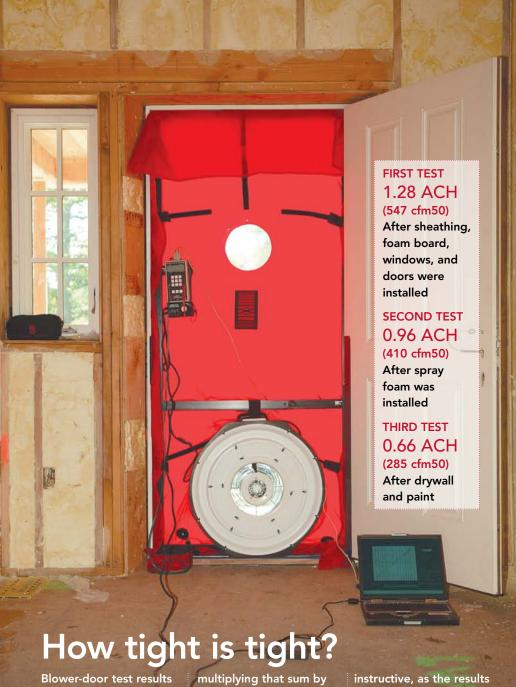
are expressed in cubic feet per minute (cfm). When measuring air leakage, this value is combined with an industryadopted standard of 50 pascals (a pascal is a
