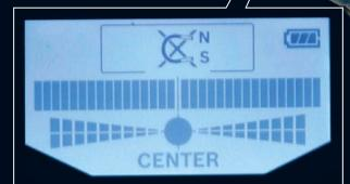
The display screen on this unit indicates the type of building material and its location. Here, the unit is indicating the centerpoint of a nonferrous (nonmagnetic) piece of metal, such as copper.
