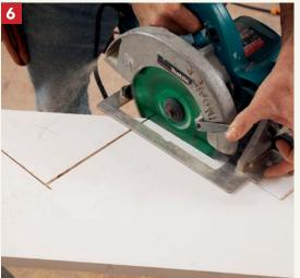
Finish with straight cuts. Cut the tread line to the miter with a circular saw. Finish the cuts with a handsaw.
