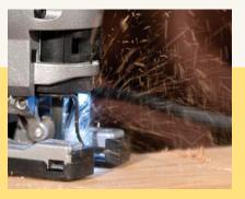
**4** ORBITAL ACTION By moving the blade in an elliptical pattern instead of just straight up and down, the cut speed increases. As speed increases, however, cut quality decreases, so this feature must be adjustable.
