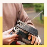
**BLADE RELEASE** You never want to grab a blazing-hot blade to remove it from the tool. Ideally, the blade can be ejected with some force or, at a minimum, can drop out easily at the push of a button.
