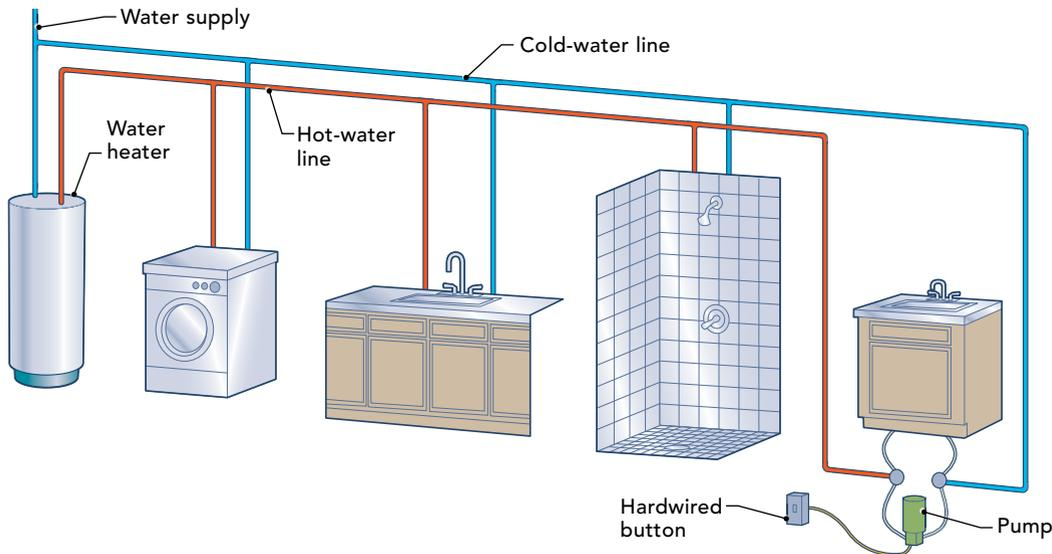
is somewhat wasteful because the pump will turn on every time someone enters the bathroom, whether or not that person needs hot water. If the house has more than one bathroom far from the water heater, it's possible to install separate switches in each bathroom, with each switch controlling the same pump.
