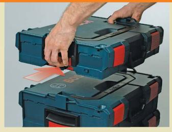
One click, but two hands. Bosch's 1-Click system allows the boxes to clip together simply by stacking them; there are no latches to operate. To separate the boxes, press a release button on each side of the box and lift. Unlike the others, these boxes require two hands to unclip and cannot be opened in a stack.
