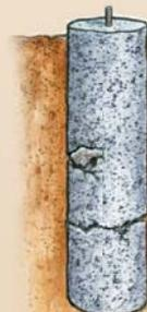
**Air pockets/cold joints:** This problem often occurs when using a stiff concrete mix, when a pour is interrupted and fresh concrete is placed on top of curing concrete, or when large aggregate doesn't consolidate into the mix. Don't pause for more than 15 minutes during each pour, and vibrate or rod the concrete to ensure that layers are intermixed.
