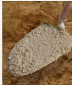
**Too wet:** Soupy concrete dilutes compressive strength. As the extra water dries away, tiny holes remain and weaken the concrete.
