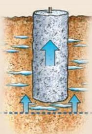
**Too shallow:** Decks connected to a house must be supported by footings that reach the frost line, the point below which the ground won't freeze. Otherwise, when moisture in the earth freezes and expands, it can push shallow footings upward. Frost depths vary, so check the local building department for your conditions.
