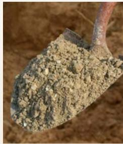
**Too dry:** A stiff, dry mix may not consolidate fully, so the footing could be left with air pockets and fracture lines that can lead the footing to crumble under load.
