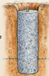
**Uneven tops:** It's hard to plumb and secure a post base properly on top of a footing with a sloped top. Make sure to screed and level off the top of the concrete before it cures.
