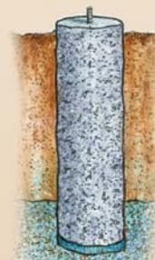
**Water infiltration:** If you hit water as you dig the footing holes or leave rainwater in a footing hole before pouring, the concrete will be contaminated and weak. Water must either be removed from the hole, or the concrete must be isolated from the water by using a plastic bag or waterproof footing form.
