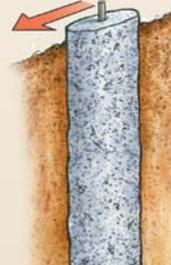
**Rocks in the mix:** Avoid the temptation to toss stones into the concrete pour. Soil on the stones will prevent the concrete from bonding, and there's also a risk of creating air pockets and weak spots.
