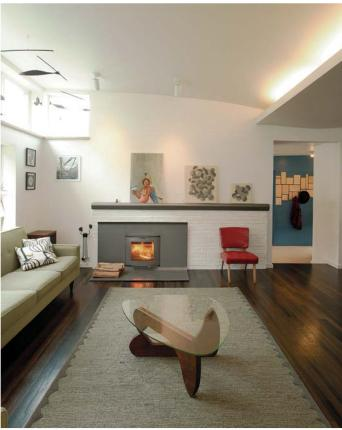
**Open it up.** The remodel raised to a curvy 12 ft. the living-room ceiling, which intersects with the kitchen ceiling at a lighted valance. A modern woodstove insert, the home's main heat source, is set into a custom steel surround.
