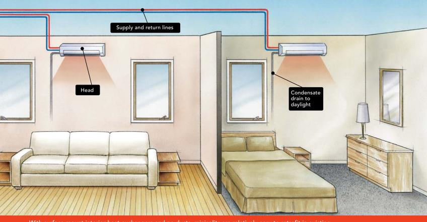
With surface-mount interior heat exchangers and no ducts, minisplits are relatively easy to retrofit in existing houses where there are no ducts. Each compressor can handle up to eight interior heat-exchanger heads, which makes zoning a simple matter. Well-insulated new homes often can be heated with a minisplit and a minimal number of heads, and efficient models can produce heat more cheaply than conventional fuel-burning systems.
