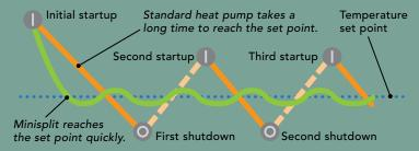
After it reaches the temperature set point, a standard air-source heat pump has to keep cycling on and off, which consumes lots of energy and results in large temperature swings.
