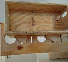
Cams support a miter-saw stand. Dowels from the cams ride in holes in the sawhorse. Rotating the cam changes its height.
