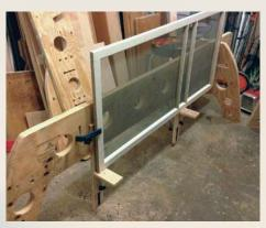
Handy hold-down. Commonly available at woodworking suppliers, a bench dog used sideways clamps a workpiece solidly.
