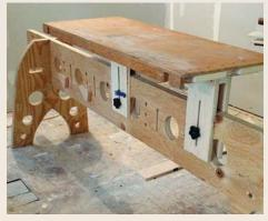
Job-site workbench. T-bolts and knobs allow the slotted supports to hold the benchtop at a variety of heights.
