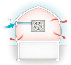
Better Supply-only ventilation is the inverse of the exhaust scenario: A fan pulls fresh air into the house; under pressure, air finds its way out of the house through cracks. This is an improvement over the exhaust-only system because pressurizing the house makes the fan less likely to pull air from the garage and because incoming air can be filtered. Depending on the system, though, it can be inefficient to use the furnace fan to distribute air.
