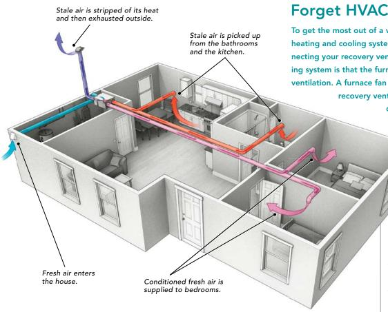
is whether they should choose an HRV or an ERV. The essential difference between the two is that an ERV transfers moisture, as well as heat, between the two airstreams. If you live in a region with a very consistent climate, then the answer is simple: Choose an HRV for cold climates and an ERV for hot, humid climates.
