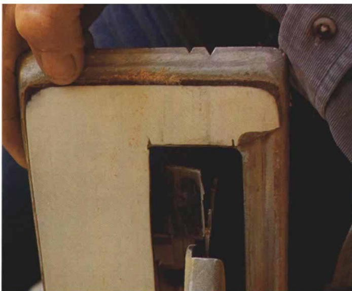
To protect fragile door skins, Royal Schieffer's saw has a piece of plastic laminate contact-cemented to its base. The bent end of the metal flange to the left of the blade holds the wood fibers in place during the cut.
