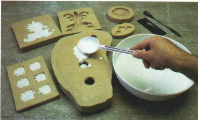
Flaharty spoons casting plaster into the two-part urethane mold of the stair-hall medallion. He's already poured a gang mold and single mold for parlor ornaments.
