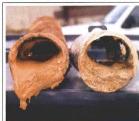
Clogged footing drains can't do the job. Water draining into the pipe carries silt that eventually fills the pipe. To avoid replacing a clogged footing drain, the author surrounds the pipe with a layered filter that stops sediment.
