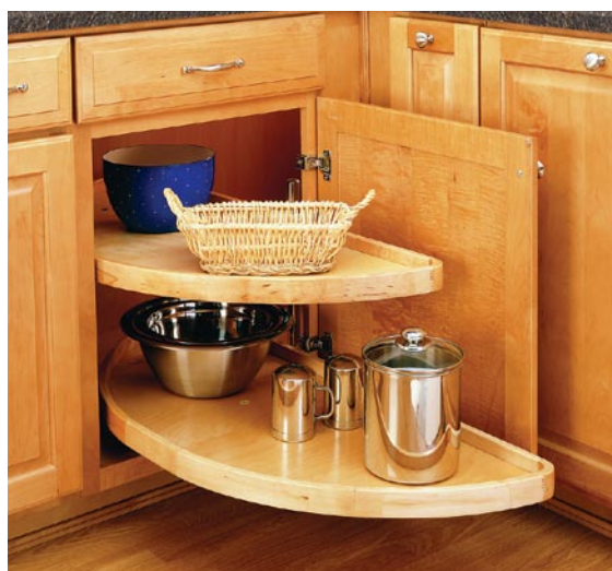
Curving around a corner. Rev-A-Shelf's Half Moon Shelves pivot and pull out of a blind corner. The 5/8-in.-thick multi-ply wood trays come sized for door openings as small as 12 in. and can be used in framed or frameless cabinets ($305-$403).
