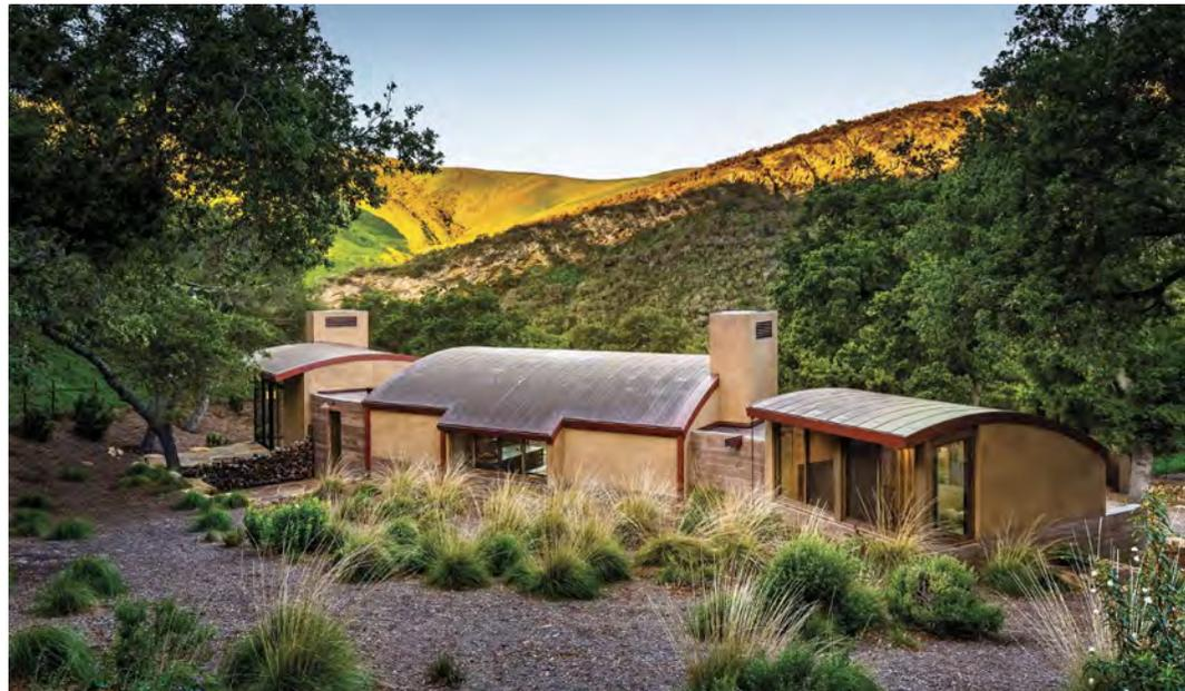
**Smoothing the seams.** The roof's copper material is low maintenance and its natural patina blends in with the scenery. A sheet-metal company was brought in to handle the seams; the goal was to achieve a soft look that would work with all of the curves. The sandstone-colored plaster emulates the eroded sandstone in the landscape.
