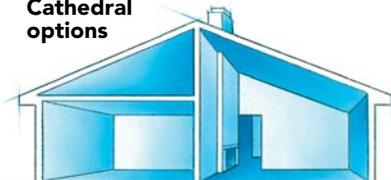
**A monoslope** ceiling extends from the exterior wall's top plate to the roof ridge.
