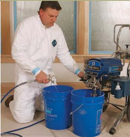
**Flush with solvent.** Fill the pump with a solvent compatible with the coating you're spraying. Spray it through the line at low pressure until it's running clear and smells clean (without traces of the previous coating or nonwater-based solvent).
