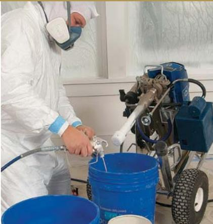
**Relieve the pressure.** Without touching the bypass valve, turn the pressure all the way down. Remove the tip and guard, and place them in a container of appropriate solvent. Slowly pull the trigger to release the pressure.
