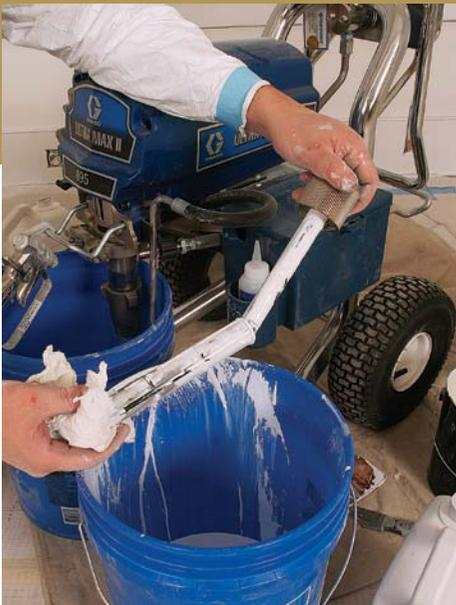
**Clean the filters.** Remove the inlet strainer, manifold filter, and gun filter, and shake them in a bucket of solvent to clean them. Reassemble the sprayer without the filters, and run solvent through the sprayer and bypass hose until it's nearly clear. You can reuse the solvent later.
