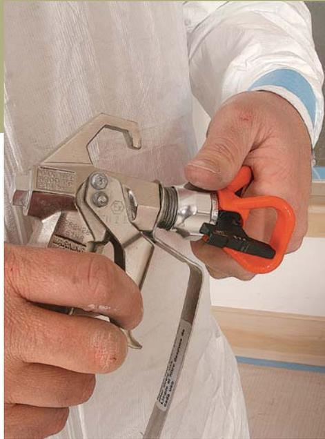
**Install the tip.** Install the tip into the tip guard so that the arrow is pointing away from the gun. Screw the tip assembly onto the gun, and align the guard to choose a vertical or horizontal spray pattern. Make the connection hand tight.
