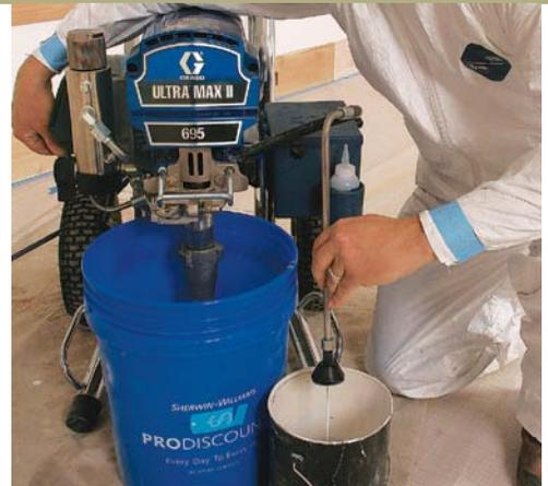
**Prime the pump.** Place the suction tube into the paint, and put the bypass hose into an empty can or bucket. Turn the bypass valve to the prime setting, and turn the pressure-control switch all the way down. Turn on the sprayer and slowly increase the pressure, but no more than halfway. When a steady stream of paint comes out of the bypass hose, turn the pressure back down to zero. Turn the bypass valve to the spray setting. The pump is now primed.
