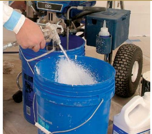
**Flush with solvent.** Turn the bypass valve to the spray position, and turn up the pressure while pulling the trigger. Aim the flow into the paint can. Once the paint is emptied from the hose and solvent starts coming out of the nozzle, move the stream to a waste bucket. Continue running solvent through the system until it's nearly clear.
