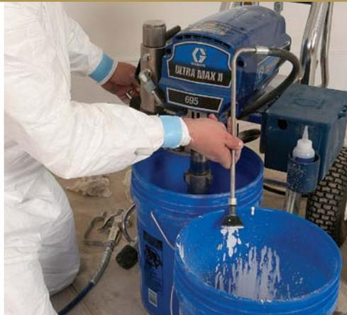
**Pump out the paint.** Place the suction tube into a clean bucket of solvent, and turn the bypass valve to the bypass setting. Slowly turn up the pressure to flush the pump with solvent. Paint will come out of the bypass tube, which can be put back in the can. Once solvent starts coming out, collect it in a waste container.
