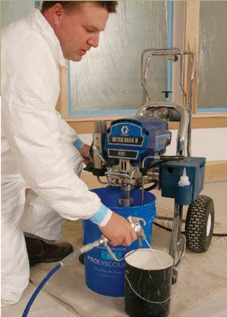
**Fill the hose.** The gun should not have the tip guard and spray tip installed yet. Unlock and pull the trigger while aiming the gun into an empty can. Slowly turn up the pressure. When a steady stream of paint starts coming out of the gun, switch the flow into the fresh-paint container for several seconds to clear air from the hose. Turn the pressure all the way down again, and lock the trigger on the spray gun.
