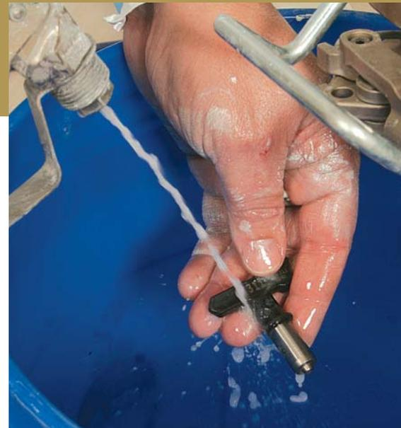
**Clean the tip and the guard.** Shake the tip and the guard in the pail of solvent to clean them. You can use a toothbrush to remove stubborn residue. Don't leave water in the sprayer in freezing temperatures and never for more than a day or two. Instead, fill the pump with RV antifreeze prior to storage to prevent corrosion and freezing.
