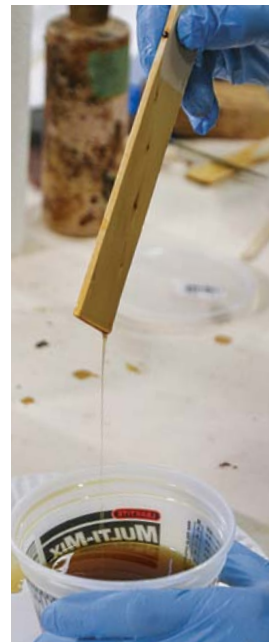
Gauge the viscosity. Let the stirred varnish run off the end of a mixing stick while counting (one-one thousand, two-one thousand, etc.). If the stream changes to drips at around the four count, you're good to go. If it takes much longer, thin the finish and test again.
