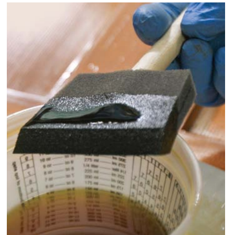
Charge the foam. After wetting the foam brush with mineral spirits, dunk it several times into the varnish, letting the finish soak into the foam between each dunk. This loads the foam with finish for a better application.
