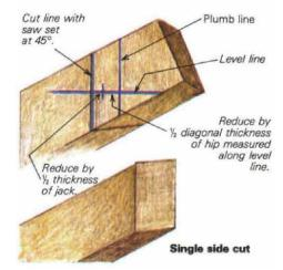
level line as shown in the illustration, above right. With a 2x hip or valley, this measures  $1\frac{1}{16}$  in. To reach the short point of the side cut, make a further reduction along the level line for one-half the thickness of the jack itself. This measures  $\frac{3}{4}$  in. The jack reduction is necessary because you are laying out the side cut on the side of the rafter, rather than on the centerline of the top edge.
