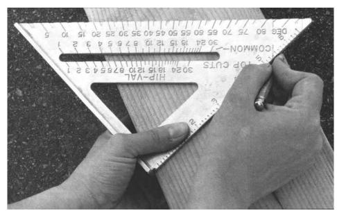
The Speed Square is an aluminum casting small enough to fit into nailbags. Angles in degrees are given on the face of the tool, and it comes with an instruction book and rafter tables.
