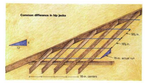
the appropriate table on your square (16-in. spacing or 24-in. spacing) and look up the pitch of your roof. The figure you see listed is the length of the first jack, excluding the length of the tail, and also the increase in the length of each subsequent jack.
