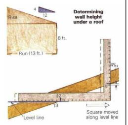
body representing a level line. Then move the square along this line until 13, representing the actual run, lines up with the edge of the material. The answer,  $4\frac{4}{12}$ , reads on the tongue of the square where it first comes in contact with the wood. This figure (4 ft. 4 in., when multiplied from unit dimensions to actual dimensions) represents the rise of the wall above the established 8-ft. mark. The height of the other wall is then 12 ft. 4 in.
