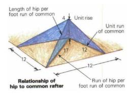
12in. mark on the body of your square to find the cuts and lengths of common rafters, you use the 17in. mark to work with hips and valleys. However, you still use the same rise figure and, in stepping off, take the same number of steps as you would with a common.
