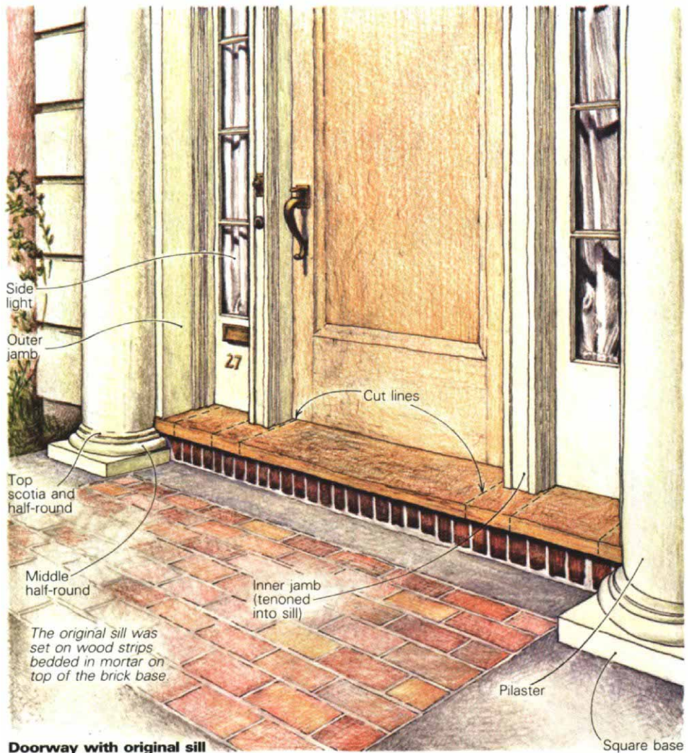
Doorway with original sill
