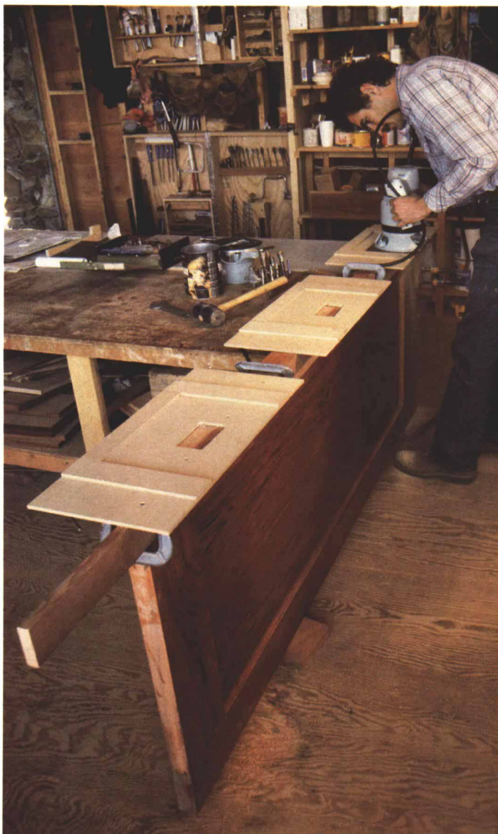
A router mounted under the wing of a table saw turns the saw table into a shaper (top left). The bit protrudes through the table, where a clamped-on wooden fence is aligned with it. At center, the author uses an ovolo bit with a fillet to carve a decorative edge on a door rail. A slot for the door panel was cut with a winged slotting cutter. The template at left is used along with a guide bushing (drawing facing page, bottom) to cut a hinge-plate mortise. As with all routed mortises, the corners are rounded and have to be squared with a chisel. Above, this template uses fences to guide the router base as the bit cuts mortises for butt hinges. The rectangular hole in the center of each template shows the area where the bit cuts. The slot in front of the stile is an entry hole for the bit.
