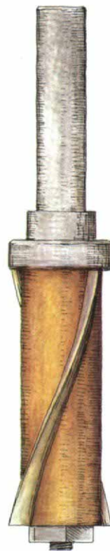
Trim bit A trim bit is used with a pattern to produce a finished surface. In the photo below, a 3-in. bit with a bearing above the cutters follows a straightedge clamped to a door.
