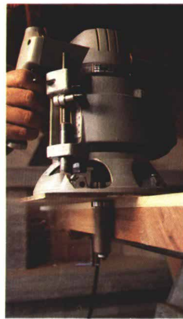
Trim bit A trim bit is used with a pattern to produce a finished surface. In the photo below, a 3-in. bit with a bearing above the cutters follows a straightedge clamped to a door.
