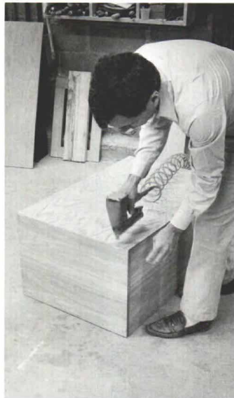
Carcass construction. Cabinet sides are daddoed to receive the rabbeted top and bottom, above. All joints are glued and gun-stapled. Levine switched to pneumatic stapling because nails and screws were too time consuming. The carcass is squared when the 1/4-in. plywood back is attached. The back has to be cut perfectly square, and after one corner is stapled down, right, the rest of the carcass is held square while the remaining sides are stapled.
