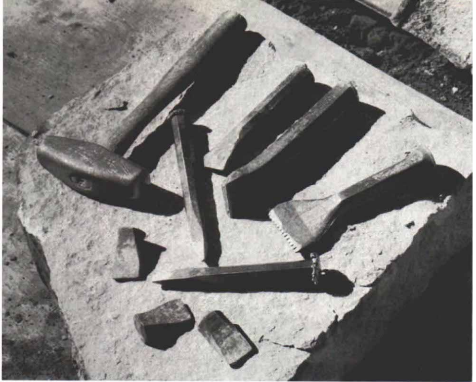
Clockwise from the top, Soto's hammer, a point, two pitching tools, a toothed chisel and a lifter. The three wedges were custom made by a blacksmith.
