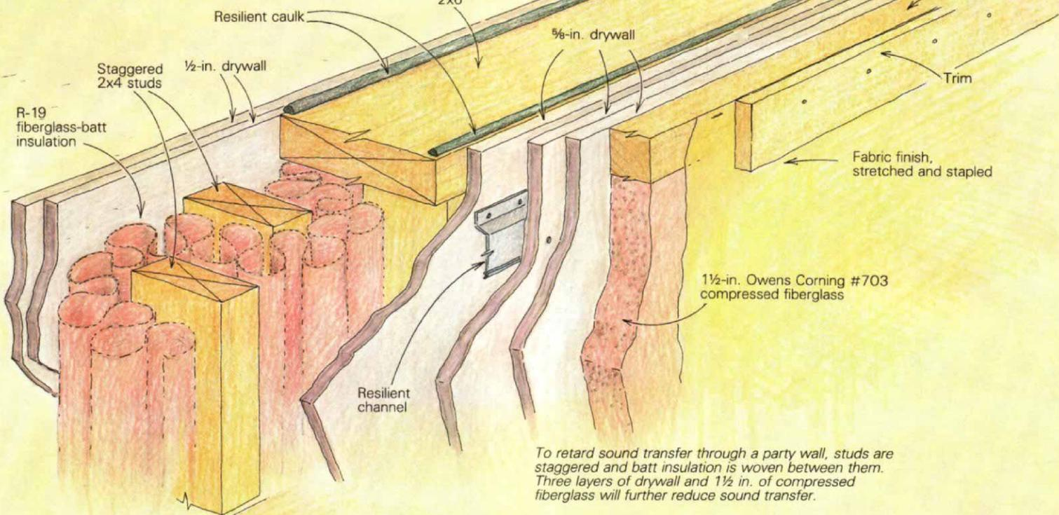
To retard sound transfer through a party wall, studs are staggered and batt insulation is woven between them. Three layers of drywall and 1 1/2 in. of compressed fiberglass will further reduce sound transfer.
