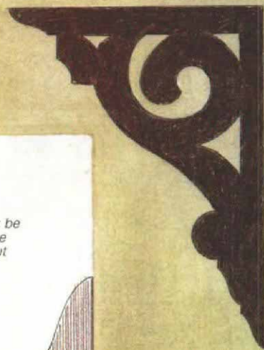
D. Brackets can be fragile because short-grain sections are liable to crack when a carpenter tries to nail them in place. To avoid this, they can be glued and nailed carefully to a partial frame. The frame strengthens the scrollwork and takes the nails when attached to the house.
