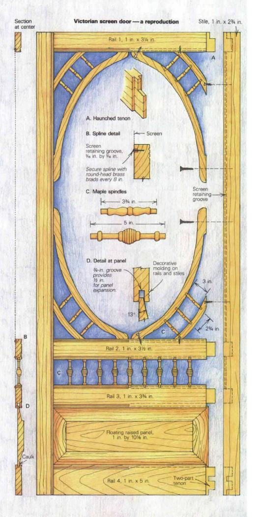
grooving plane, but this old tool is hard to come by. A series of passes over the angled blade of a table-saw will achieve a similar effect, or you could use a router. But to avoid weakening either the mortises or the groove for the panel, run the pattern to a depth of only  $\frac{1}{16}$  in.
