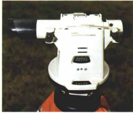
While the latest levels and transits (such as this model LT8-300 from David White) have become more streamlined, their functions remain the same as their ancestors.
