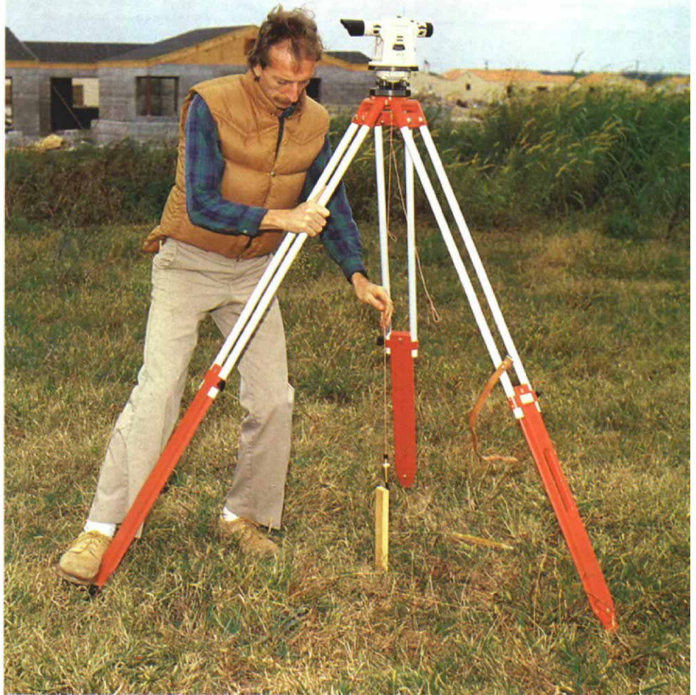
Setting up the tripod. Begin setting up a level or a transit over a fixed reference point, such as a stake, by spreading the tripod legs equally and pressing their tips into the ground. As you position the tripod legs, watch the instrument—you want it eventually to end up above the stake.
