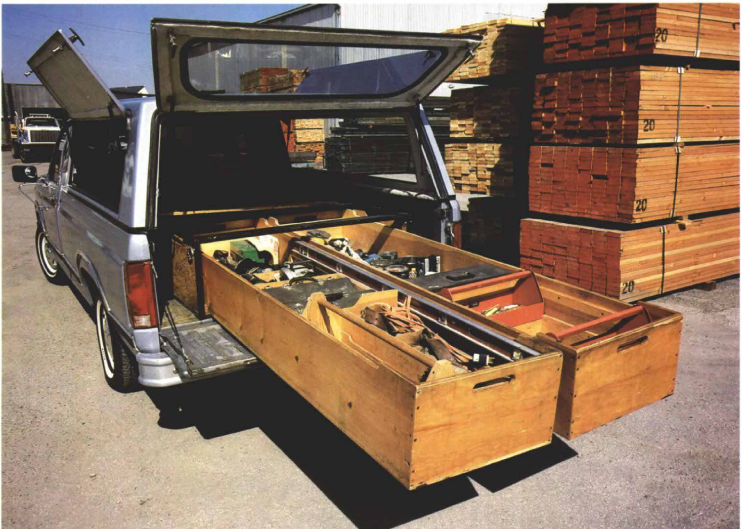
Lincoln's pickup-truck storage system consists of two 8-ft. drawers that ride in a steel and plywood carcass. Here the drawers are fully extended, with their inboard ends bearing on the second steel crossbar. The drawers are divided into compartments for related tools, hardware and supplies. Four plywood lids atop the unit make a flat surface for carrying cargo. The carcass stays put between the wheel wells without mechanical connections.
