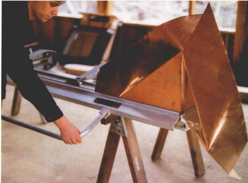
**Most of the folds were made on the metal brake shown above. Eventually the configuration of bends prevented the roof sheet from slipping into the brake, so the final folds were handmade.**
