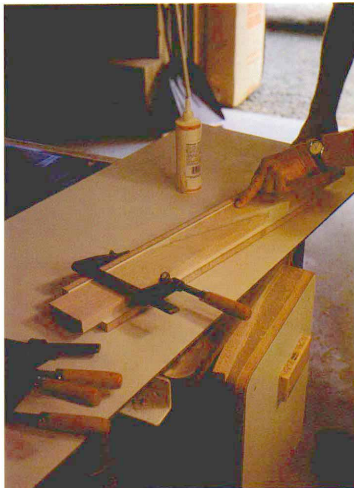
An assembly jig (photo above) assures alignment of the scarfed pieces so that the resulting joint will be nearly invisible.
