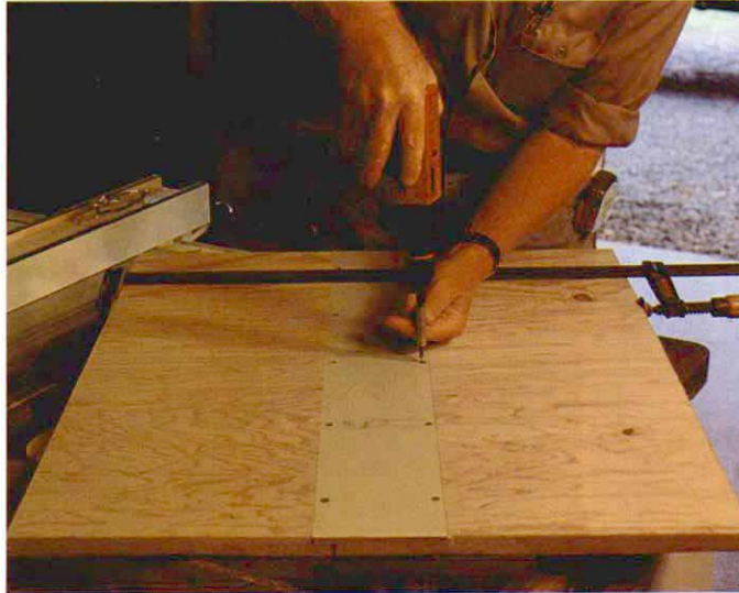
Though the base of the sliding table can be made from a single piece of plywood or particleboard, the three-piece base shown here (photo above) ensures a precise kerf line. The joint between the pieces can be seen in the foreground. Screws should be countersunk.
