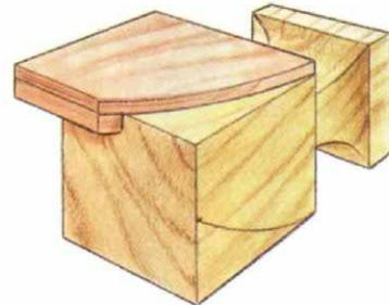
**4. Cut each arc, using a stiff blade on the bandsaw (I like a 1/2-in. blade); use a push stick to keep your hands away from the blade. Stop the cut at the tick mark and back the blade out. Turn the block 90° and cut each of the remaining sides. Separate the pieces. If you want to, sand out any "washboard" from the handsaw, but don't be too fussy—a finely sanded cap looks out of place on most decks.**
