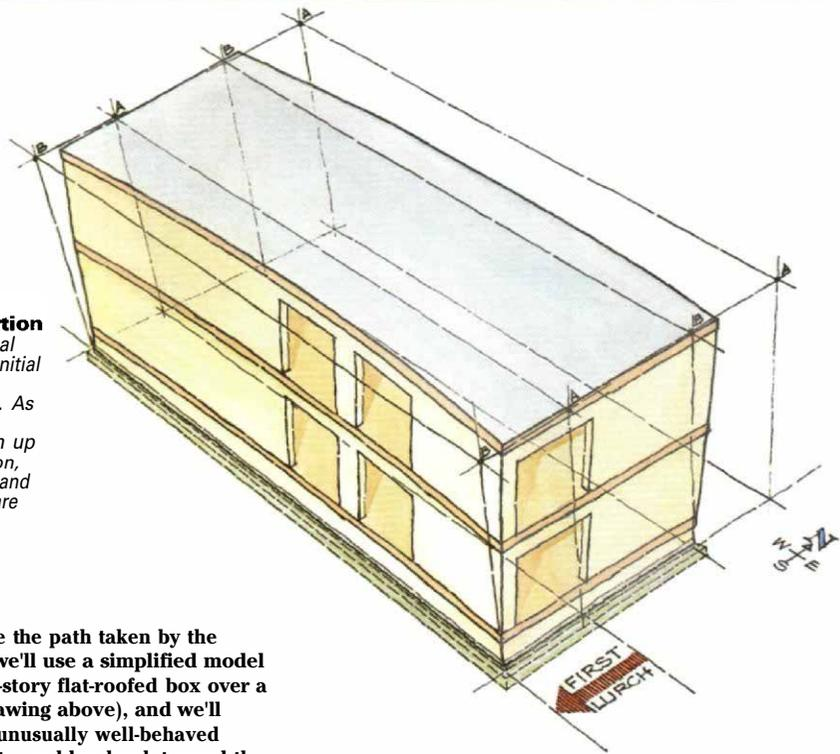
To help visualize the path taken by the inertial forces, we'll use a simplified model building—a two-story flat-roofed box over a crawl space (drawing above), and we'll subject it to an unusually well-behaved earthquake: first a sudden lurch toward the south, followed by a sudden lurch back to the north. Period. We'll start at the bottom of the building and go up, concentrating on primary effects.
