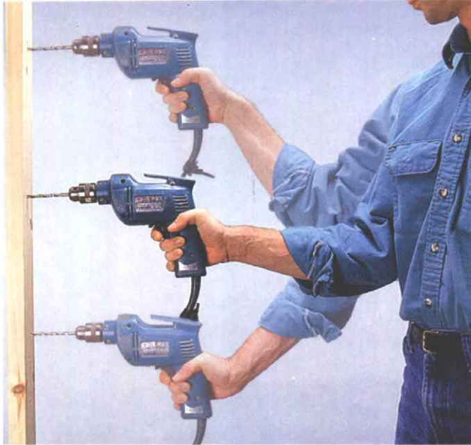
Carpal tunnel syndrome, an inflammation of the nerve at the base of the palm, is caused by repetitive gripping with the wrist bent. To help prevent it, get in the habit of using power tools with the wrist in neutral. The neutral position is naturally assumed by the wrist when you let your arm fall to your side—not bent too far in any direction. The center view in both photos shows the correct position.
