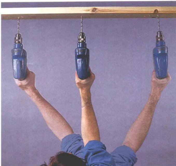
Carpal tunnel syndrome, an inflammation of the nerve at the base of the palm, is caused by repetitive gripping with the wrist bent. To help prevent it, get in the habit of using power tools with the wrist in neutral. The neutral position is naturally assumed by the wrist when you let your arm fall to your side—not bent too far in any direction. The center view in both photos shows the correct position.
