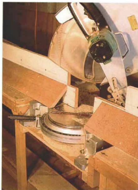
Dropped platform. The wing tables are joined by a saw platform lowered far enough to bring the saw's table flush with the wings. The fences are braced from behind with triangular blocks on 1-ft. centers.
