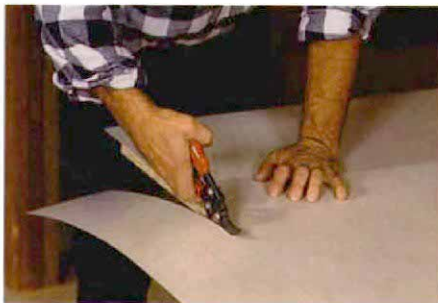
Shear force. Laminate shears, made by Klenk, have three blades—one above, two below—that remove a 1/8-in. strip of laminate. Cutting laminate with shears is faster and more convenient than cutting with a scoring tool.
