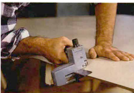
Cutting strips with a slitter. Made by Virutex, this laminate slitter can either be pushed or pulled along a sheet. Its adjustable guide allows you to cut strips anywhere from -in., to 3 -in. wide.
