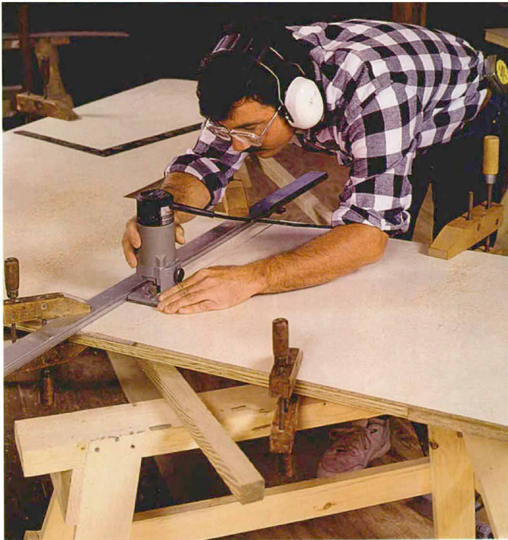
Cutting a seam. Although you should avoid seams in laminate whenever possible, sometimes you can't. Mirror-cutting is the way to get the best possible fit between two pieces. To do it, butt the pieces together temporarily and make a router cut through the middle of the seam.
