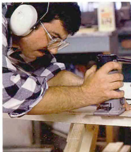
It's not a ball-bearing bit. A ball-bearing bit can seize and burn the laminate. That's why the author prefers a self-pilot bit. To avoid burning, he lubricates the guide surfaces with petroleum jelly before routing.
