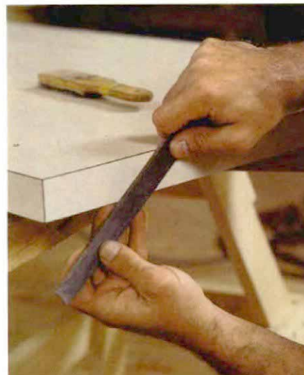
Flush-trimming bits don't trim flush. You have to file the laminate top flush by holding the file almost flat to the front edge and stroking downward. You know you're done when the excess glue at the seam shaves off, revealing a crisp, clean edge.
